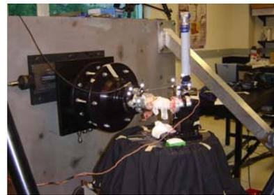
Figure 1. Rotobot Testing Platform - joint mounted
